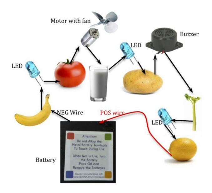
\*NOTE: "The LED (Light Emitting Diode) produces light from electrical power. To work, it has to be oriented properly (this is called polarity). Usually the two leads are different lengths. The longer lead goes to the positive, or red, side of the battery pack. The shorter goes to the negative, or black, side of the battery pack" (Squishy Circuits).
